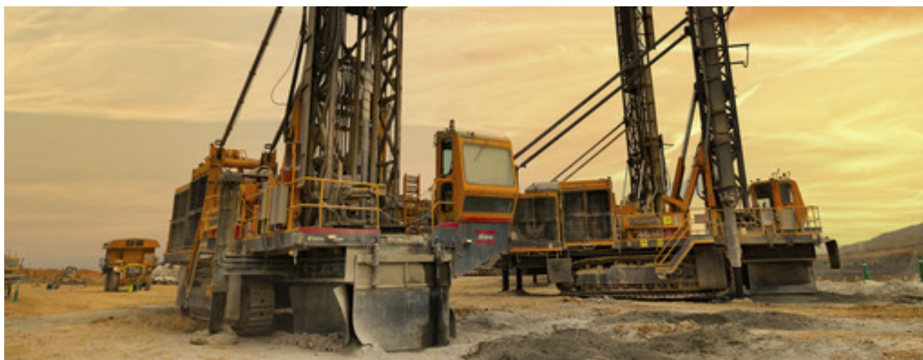
Bremote drills at Anglo Platinum's Mogalakwena platinum mine in South Africa drilling a pattern of holes for blasting at the open pit operation.
